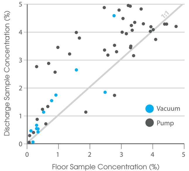
Two full-scale SedVac pilot tests were performed comparing settled solids collected at point locations on the tank floor to corresponding discharge composite samples. In both vacuum and pump configurations, Figure 2 shows that SedVac removed settled solids at concentrations greater than the intake on the basin floor. The study suggests that the shape of the header wing funnels solids toward the pump or vacuum intake, concentrating the sludge and thus increasing the discharge concentration.
