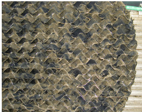
Figure 9 PVC structured sheet media with healthy biomass
