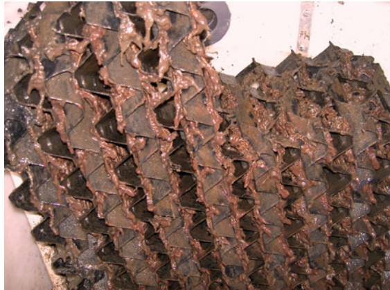
Figure 8 Excessive red worm growth on the fabric media
